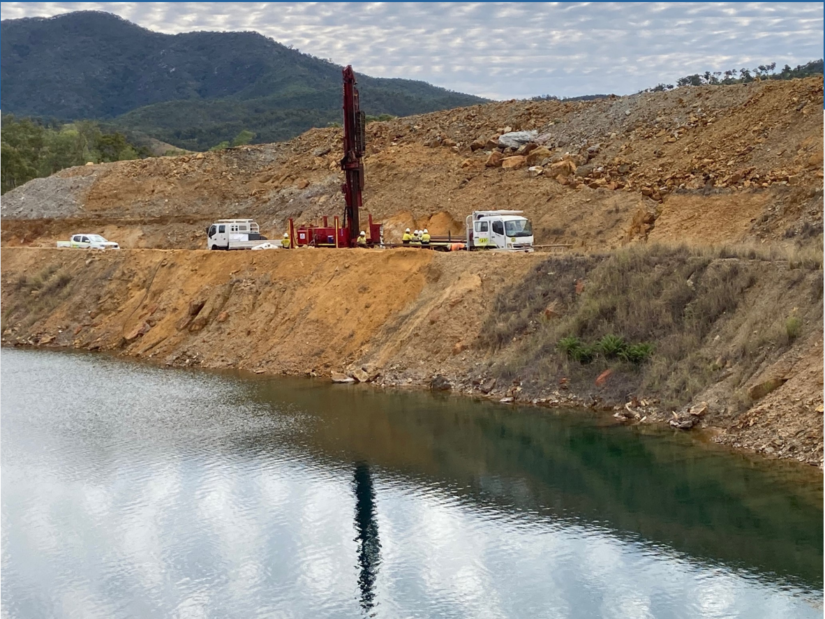
Figure 1: Diamond drilling at the west load of the flagship Mt Chalmers project.
