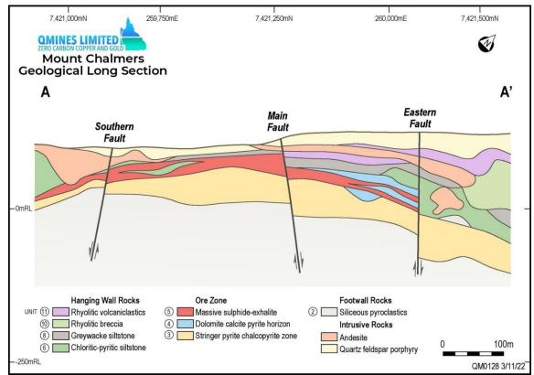
Figure 5: Mt Chalmers Geological Long Section AA'.
