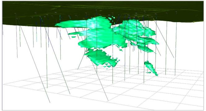
Figure 16: Woods Shaft Inferred Resources Block Model for Copper Cut Off of 0.3% Cu (Oblique View: Looking Azim 23 330, Dip -5 Degrees – Grid Shown 50m x 50m).
