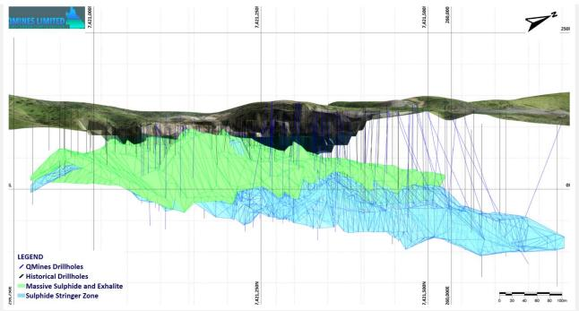
Figure 8: QMines wireframing of the Mt Chalmers mineralisation zones. Long section looking WNW.
