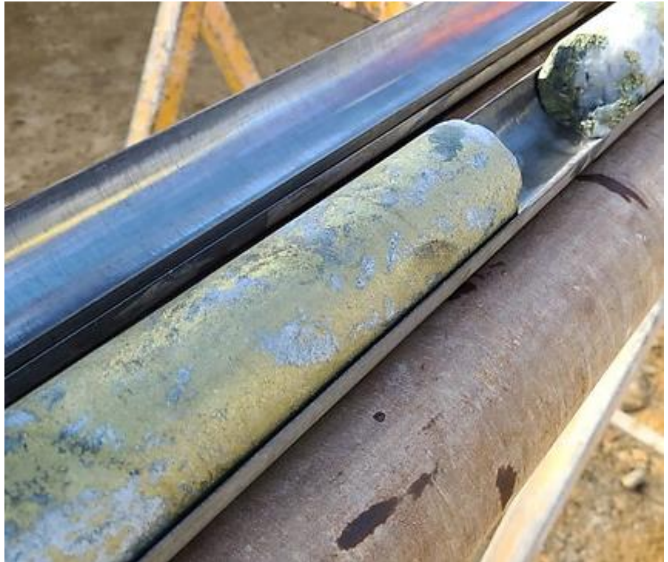
Drill Hole MCDD015 Showing Semi Massive Chalcopyrite Stringer Veins Drilling Intersects New Mineralisation Outside Resource 25 August 2021.
