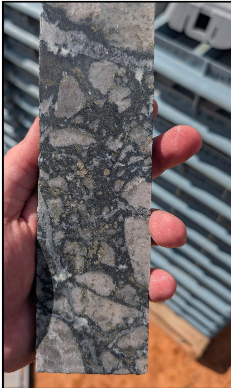
Figure 7: Representative drill core from MMDD007 (171m), mineralised enargite-pyrite hydrothermal breccia within vuggy residual quartz. Pale silica altered clasts are cemented by dark sulphide enargite rich matrix with abundant brassy pyrite. Photo: QMines.
