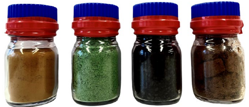
(L-R): Crushed ore, Ni-Co MHP, Hematite, Inert Residue for Landfill
