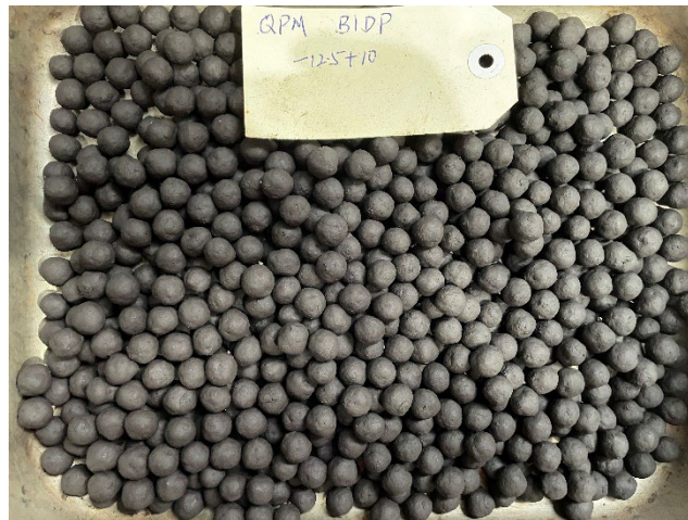
Image: Sinter pellets production from QPM iron hydrolysis hematite
