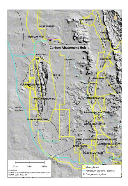
Geological formation of these deposits results in high methane gas content. Pre-mine drainage, capture and beneficial use by industry and to generate energy reduces fugitive emissions of methane, significantly lowering the greenhouse gas intensity of coal mining in the region.
