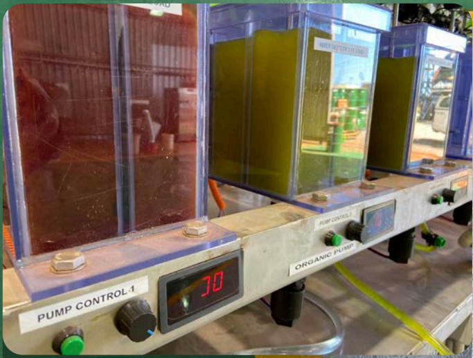
Solvent extraction process.
