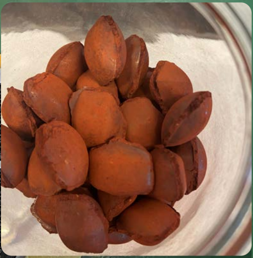
DR Grade pellets produced from red mud waste.
