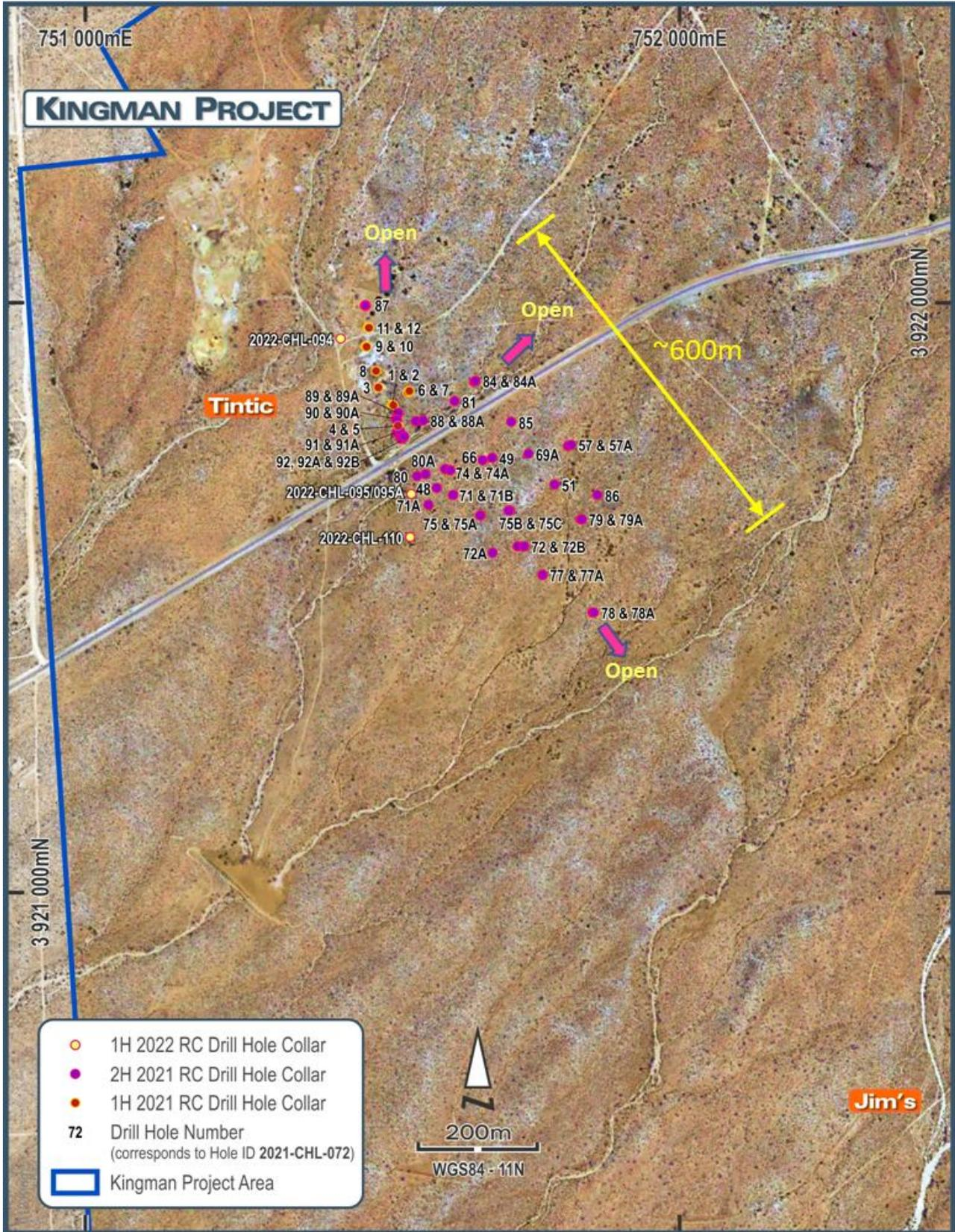
Figure 2 – Collar locations of RC drill programs over the Tintic area showing holes 095, 095A and 110 further extending gold and silver mineralisation.
