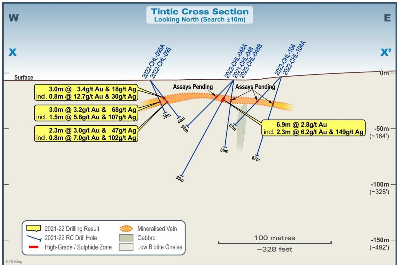
Figure 1 – Tintic Cross Section X-X'
