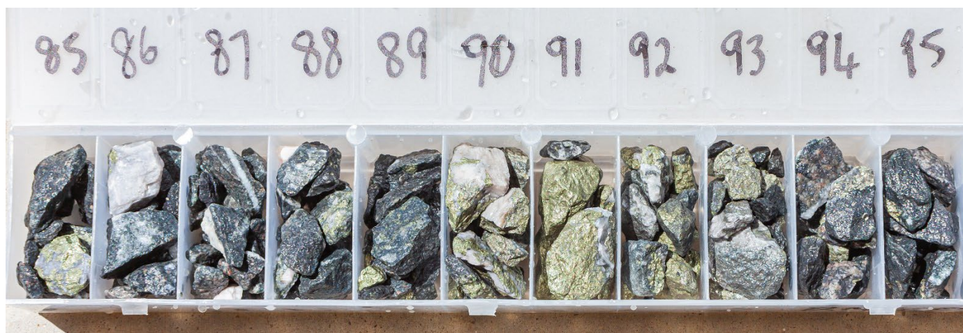
Figure 2. Chalcopyrite-pyrite sulphide zones at Mongoose - Hole RMG021.
