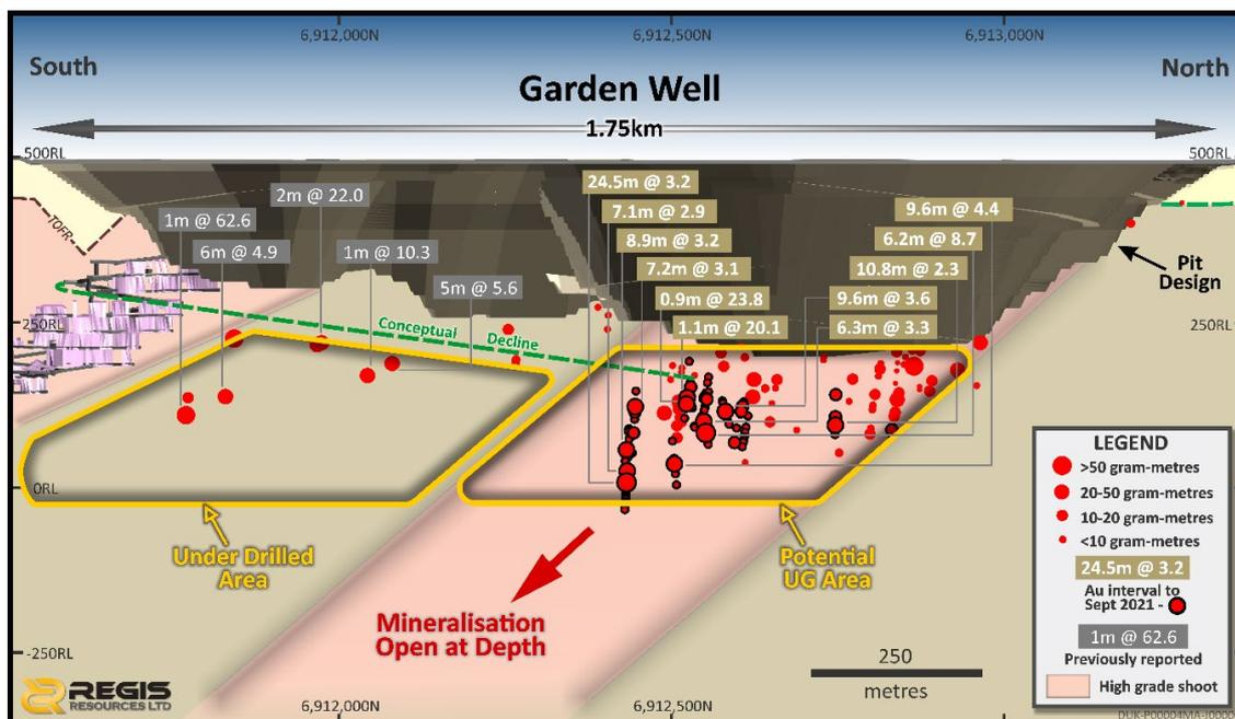
**Figure 3:** Garden Well long section looking west showing high grade intercepts under Main pit, the existing and planned underground mine at Garden Well South and the conceptual exploration decline.
