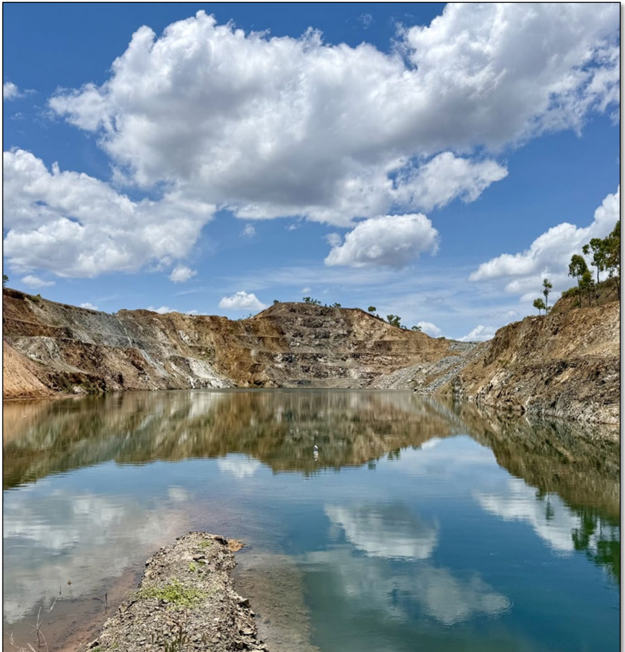
Figure 7. Willett's Pit (looking south-east) was primarily mined for magnetite. High-grade zinc mineralisation is located in the southern pit wall (left) and beneath the pit floor.
