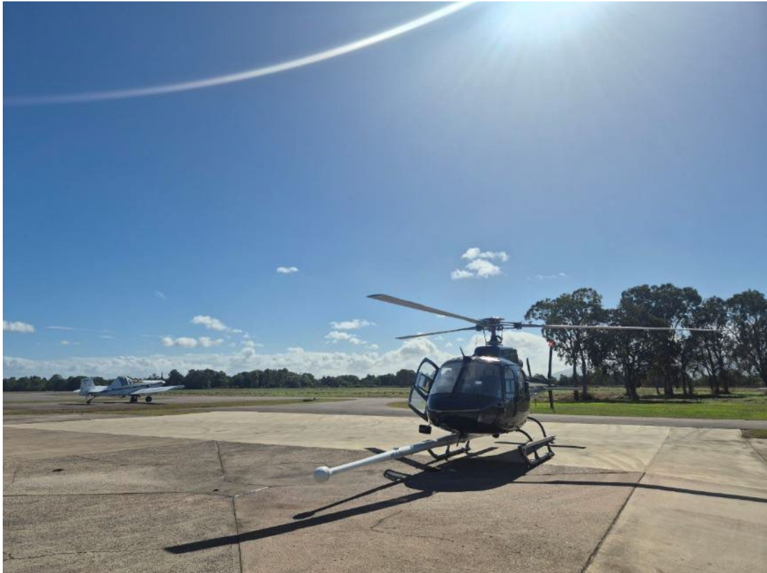
Figure 1: Helicopter with magnetometer stinger at Ingham, northeast Queensland.
