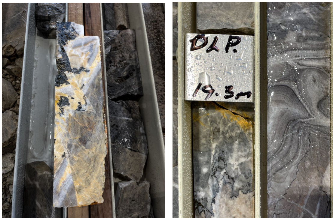
Figure 5: Mineralised Linda core DLP1 – Coarse sphaerite karst Infill (left) and stylolite vein sphaerite with karst infill (right).
