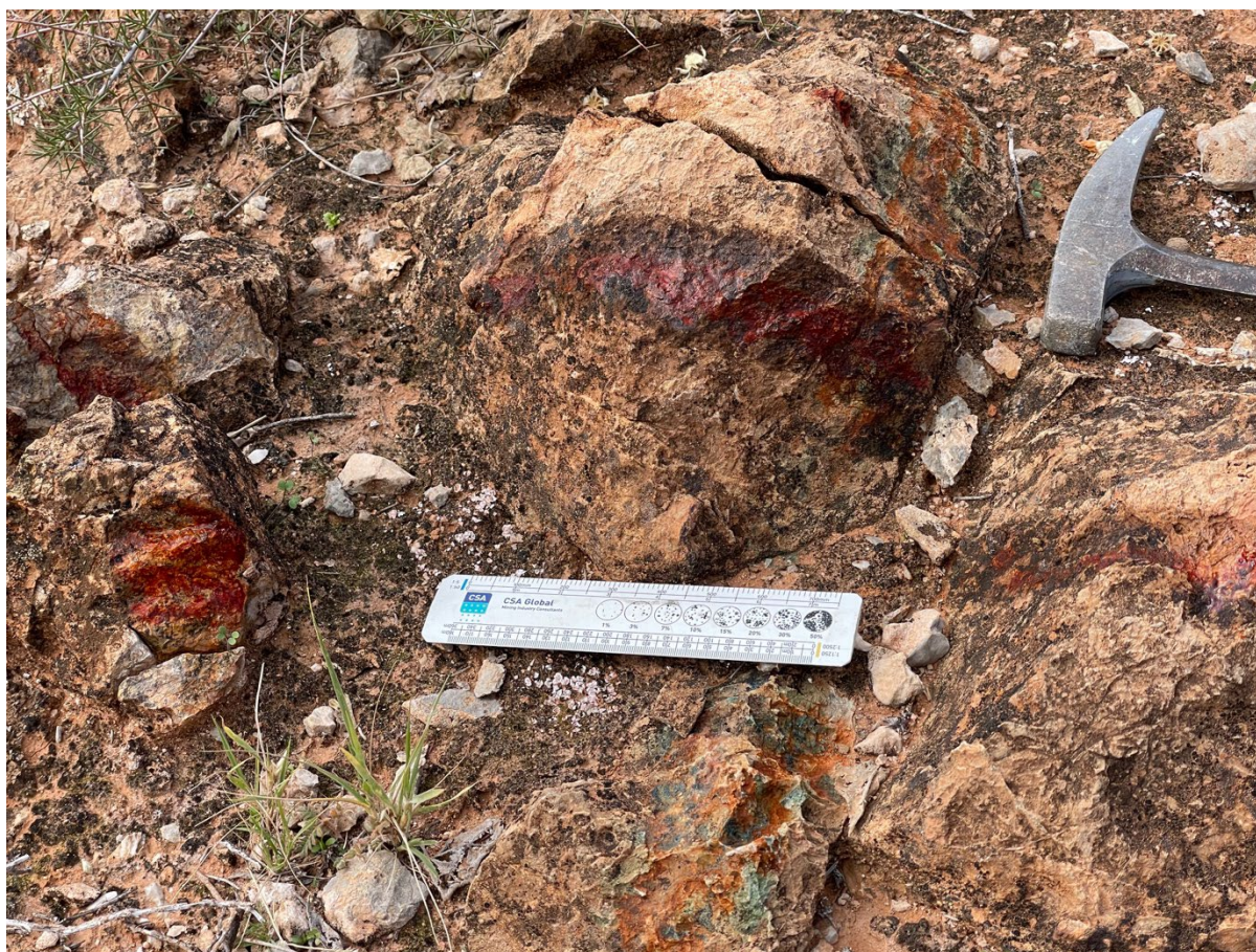
Figure 4: Example of high-grade zinc outcrop stained with zinc-zap (red indicates the presence of high-grade zinc).
