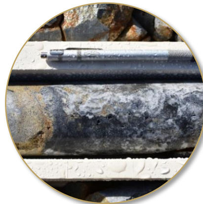
Discovery Hole BHD006. 259.5m Banded quartz, yellow-red sphalerite, galena, and MnO after rhodochrosite.
