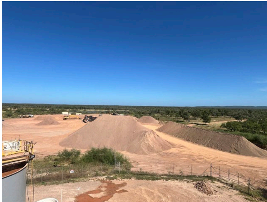
Figure 2: Stockpiles of Crushed Big Ben material on GGPP ROM pad
