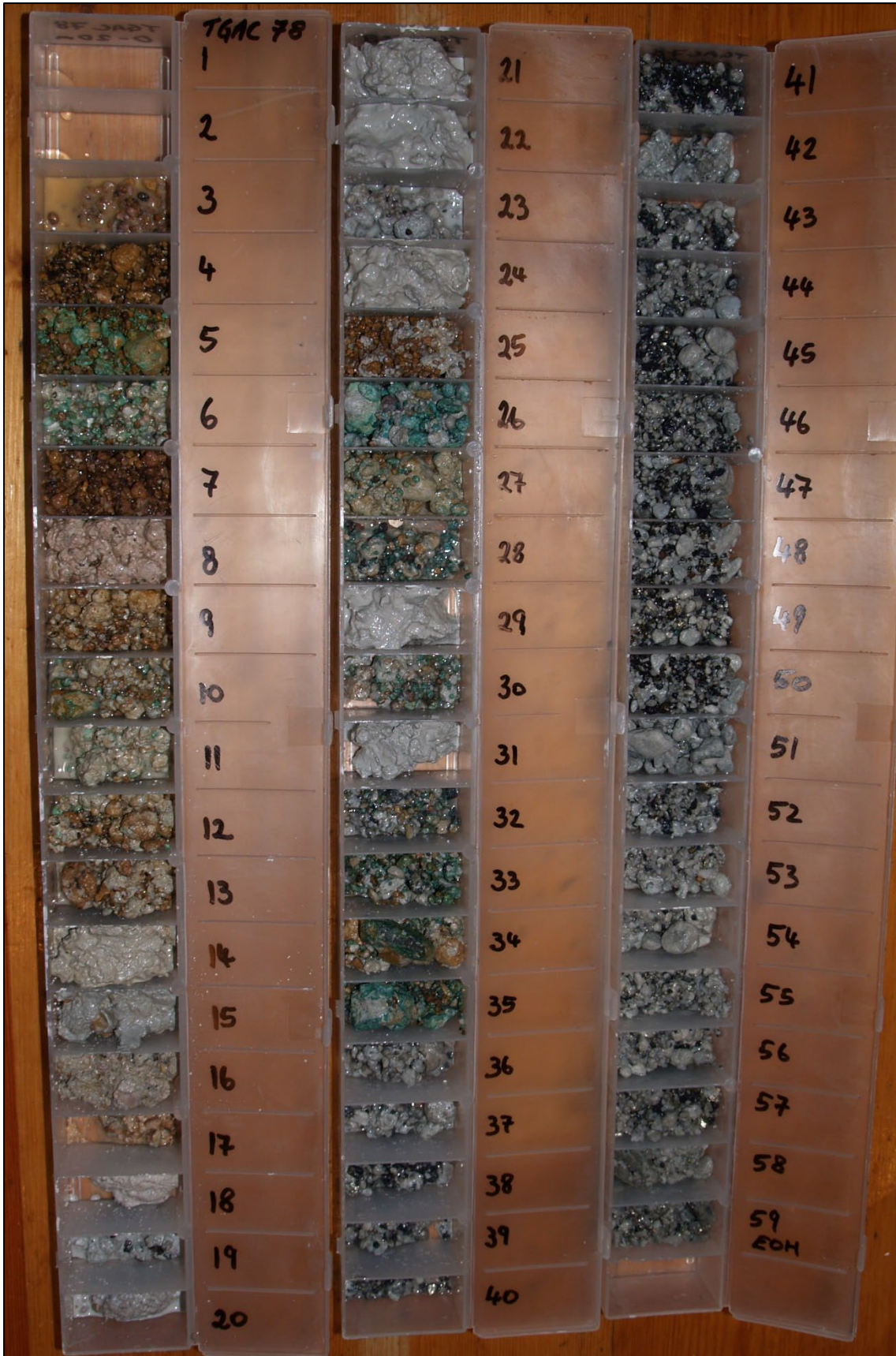
Photo 2. Percussion chip trays for aircore drill hole TGAC078. Note the green copper oxide minerals transition to fresh sulphide minerals pyrite, chalcopyrite and bornite from around 36m drill depth.
