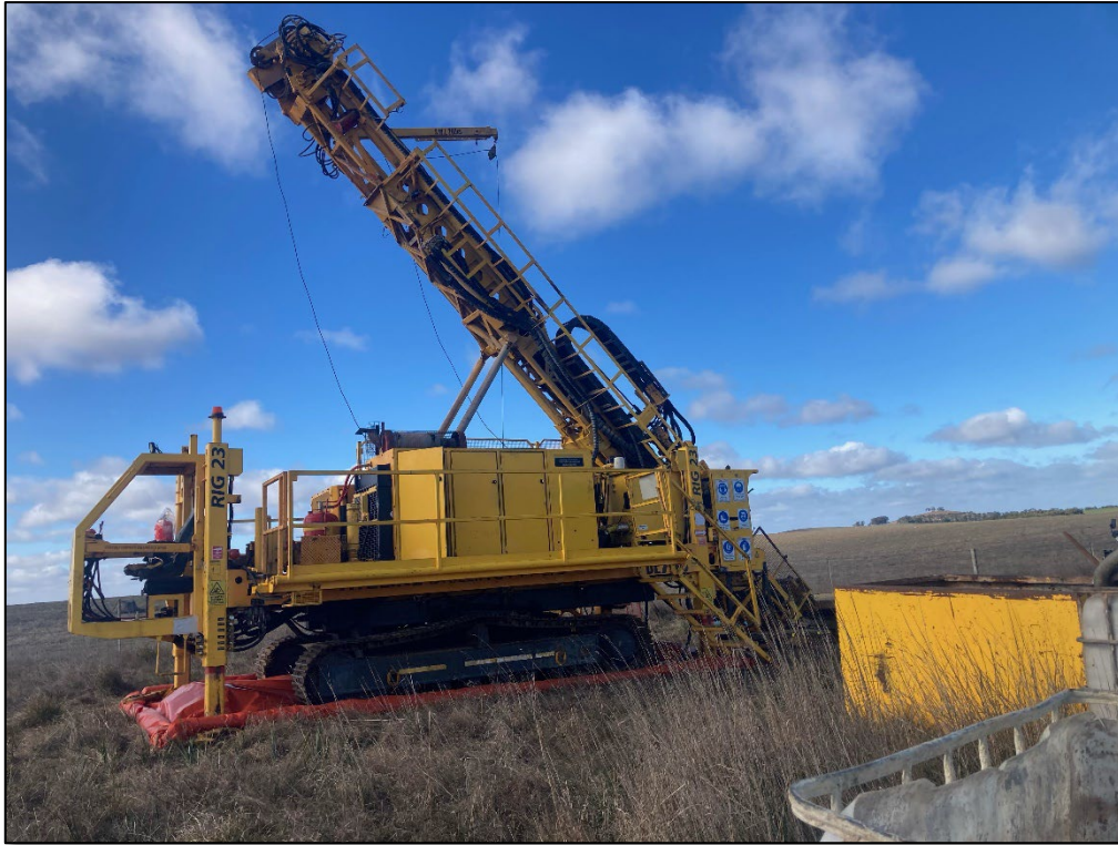
Photo 1. Diamond drill rig set up to test the Junction Lode.
