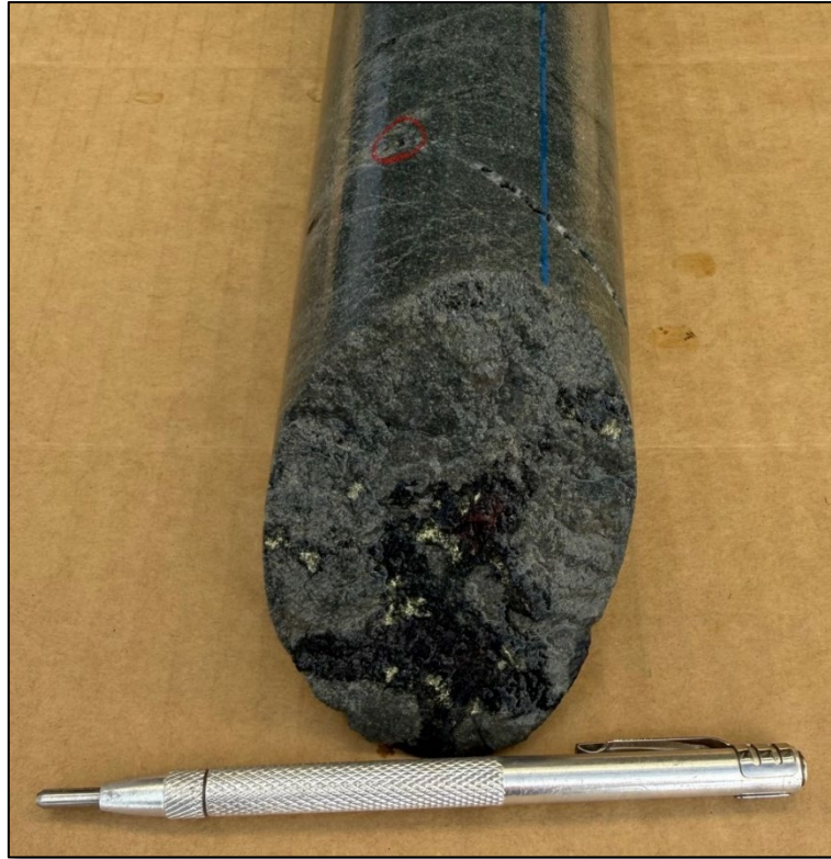
Photo 2. Chalcopyrite, chalcocite and hematite in a vuggy quartz vein at 169.2m in SJD001.
