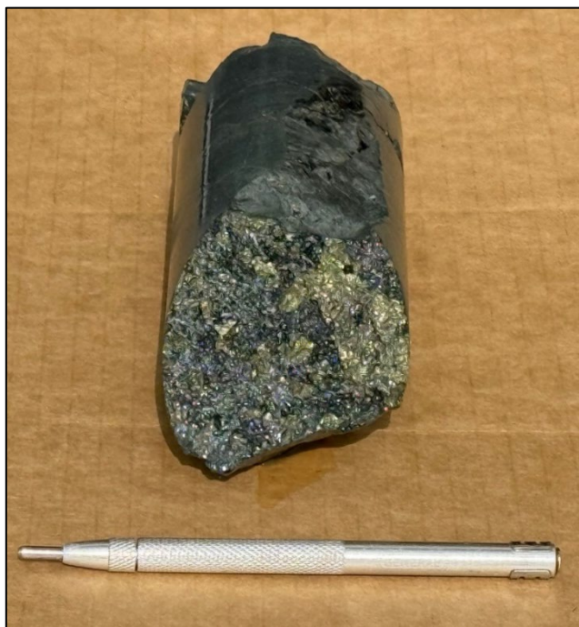
Photo 1. Chalcopyrite, chalcocite and minor pyrite in vuggy quartz vein at 160.7m in SJD001.
