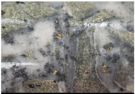
SDDSC091 from 439 m (within assayed interval 0.5 m @ 1,497.4 g/t AuEq (1490.0 g/t Au, 4.7% Sb) from 438.8 m to 439.3 m showing cut core with brecciated dioritic dyke, with stibnite and quartz-carbonate veining with fine, disseminated frequent visible gold. Millimetre scale.
