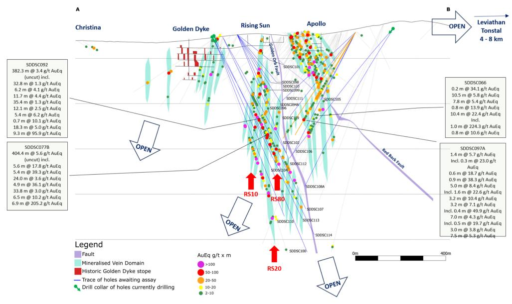
Figure 5: RS10 vein set defined at a 25 m x 50 m spacing extending over 570 m down dip and 30 m – 40 m along strike, with a 2 m @ 1 g/t Au lower cut-off grade. Drill density only limits extensions in all directions.
