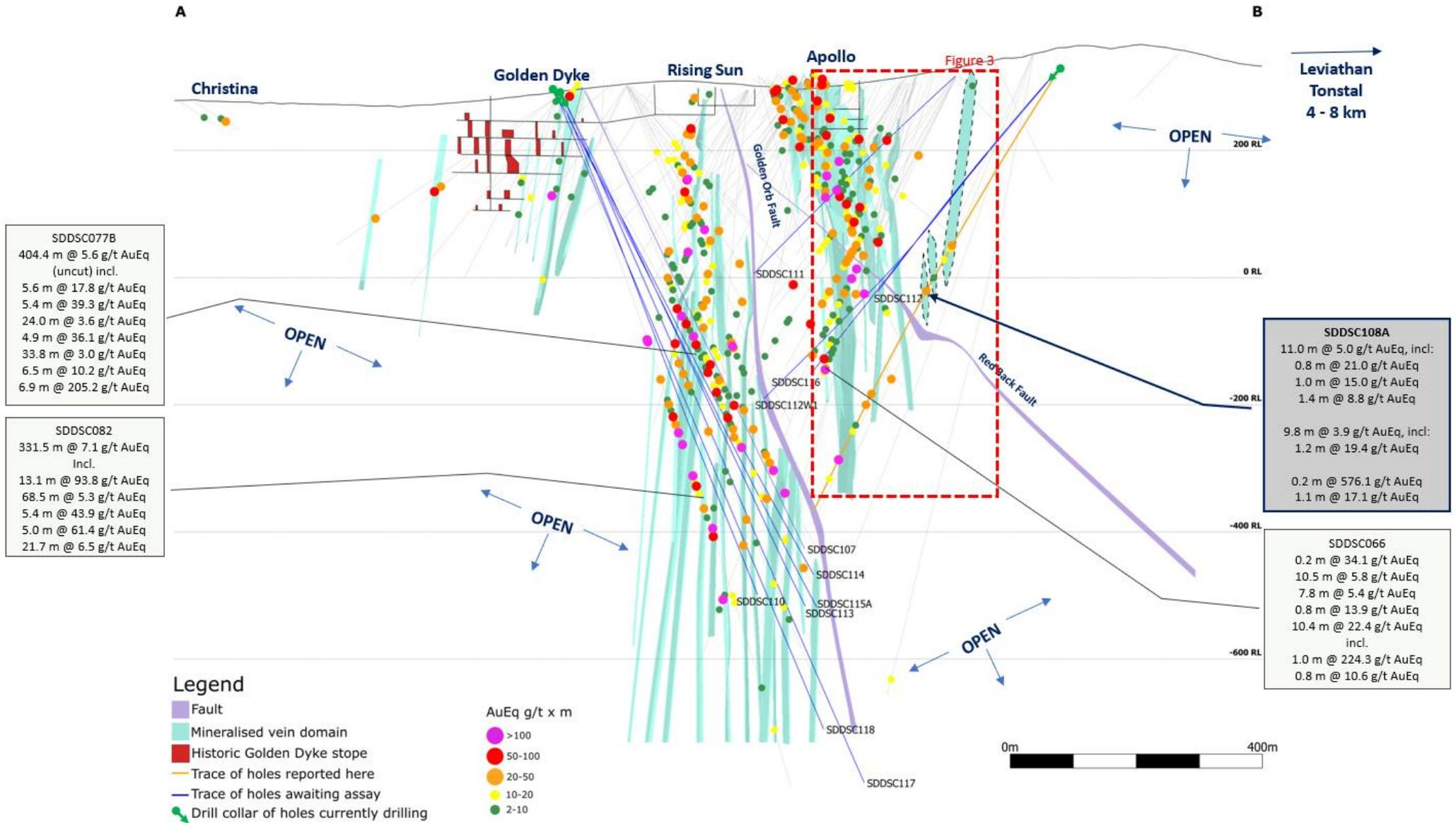
Figure 3: Sunday Creek cross section across C-D in the plane of drillhole SDDSC108A, looking towards the north (striking 092 degrees). Showing SDDSC108A (orange trace) reported here and prior reported drill holes. Section influence is 50 metres.
