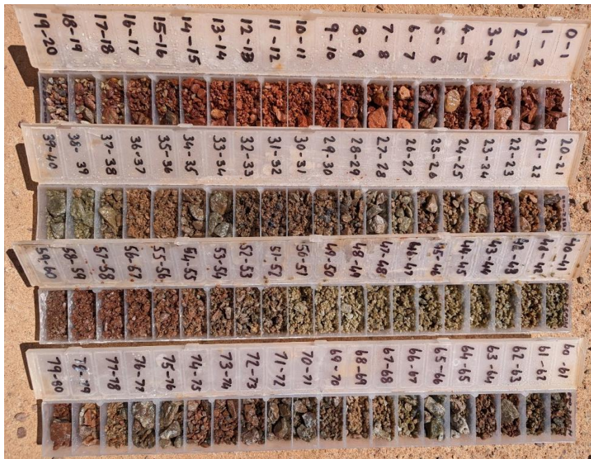
Figure 5. Chip trays from hole HRC23-008 illustrating areas of propylitic alteration (green minerals) within quartzite from 18m to 79m.
