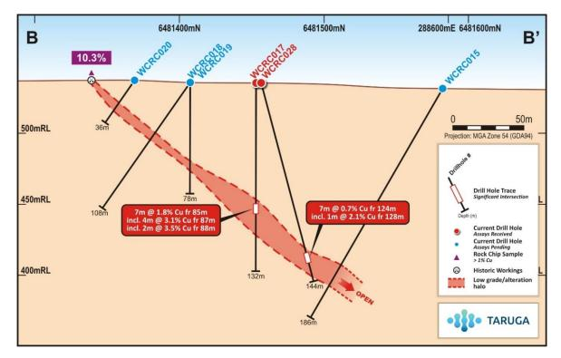
**Figure 6**. Cross Section B-B' Showing Best Intercepts, the Target Unit Outline and Rock Chip Highlight from Historical Workings.
