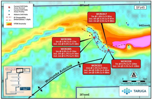
**Figure 3.** Image of the Vertical Component dB/dt Amplitude for Window 45 – 7.036 mSec, Highlighting 7km Late Time VTEM Anomaly, with an Intensified 2km x 1km VTEM anomaly in the east, which remains open along strike beyond the survey limits.
