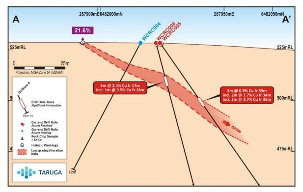
Figure 5. Cross Section A-A' Showing Best Intercepts, the Target Unit Outline and Rock Chip Highlight from Historical Workings.
