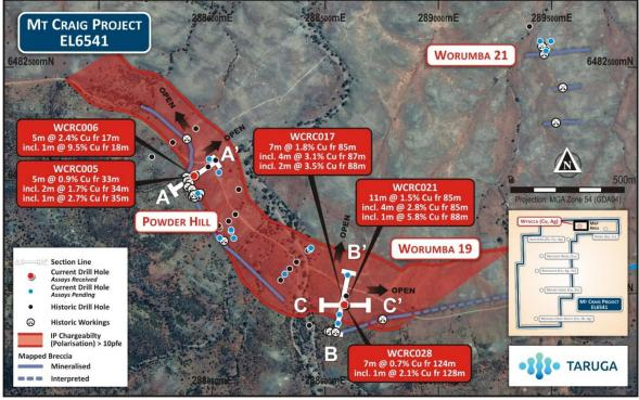
Figure 4. Plan View of the Wyacca Drill Results Showing Best Intercepts and IP Chargeability Anomaly.
