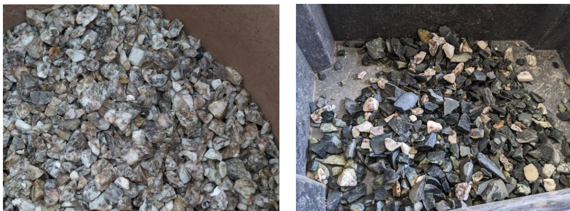
Figure 4 – Typical ore sorter products, pegmatite on the left to ore feed and basalt, feldspars and quartz on the right to waste. The photographs are of samples generated in-train and are therefore incomplete. Assays of the final products for each composite sample run are shown in Table 4.
