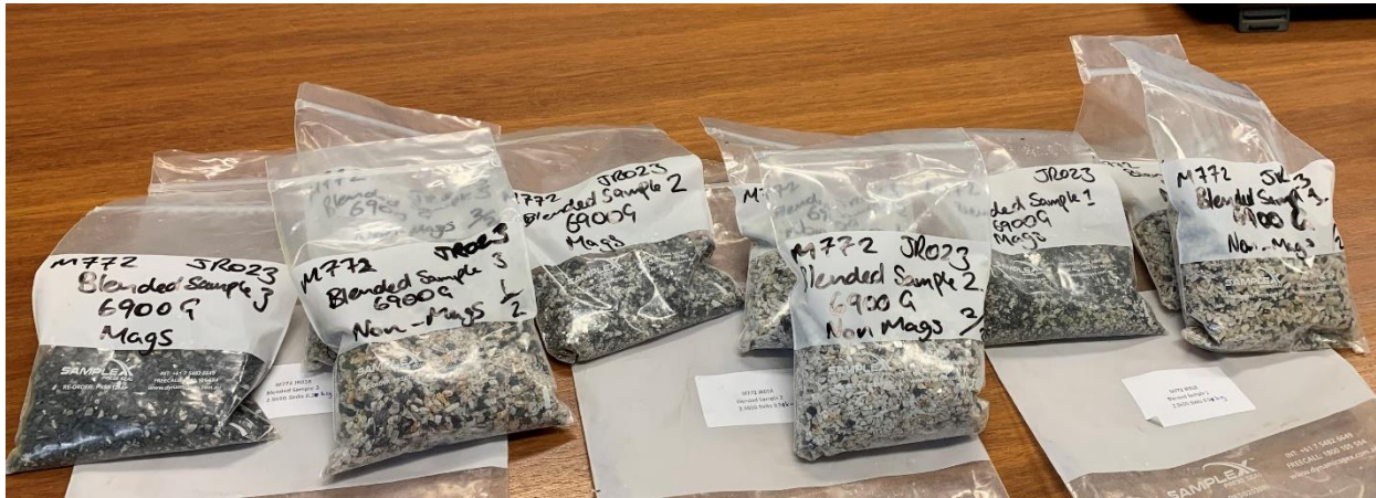
Figure 1 – HLS testwork products on 3 blended composites post magnetic separation. Non-Mags = Spodumene concentrate, Mags = Basalt, mica and feldspar Waste (Gangue). Note: the assays for these samples are shown in full in Table 5.
