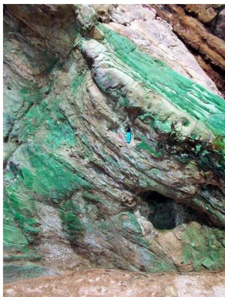
Figure 1: Face of the historic Kapunda Stockyard Pit showing distinctive oxidised copper mineralisation on the face.
