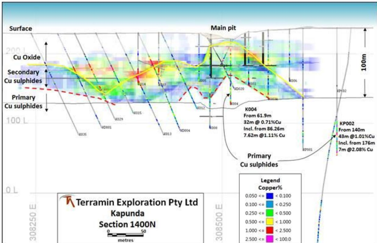
Figure 6. Kapunda cross section 1400N (looking north) showing drillholes and block model coloured by copper grade and historic workings (25m window).
