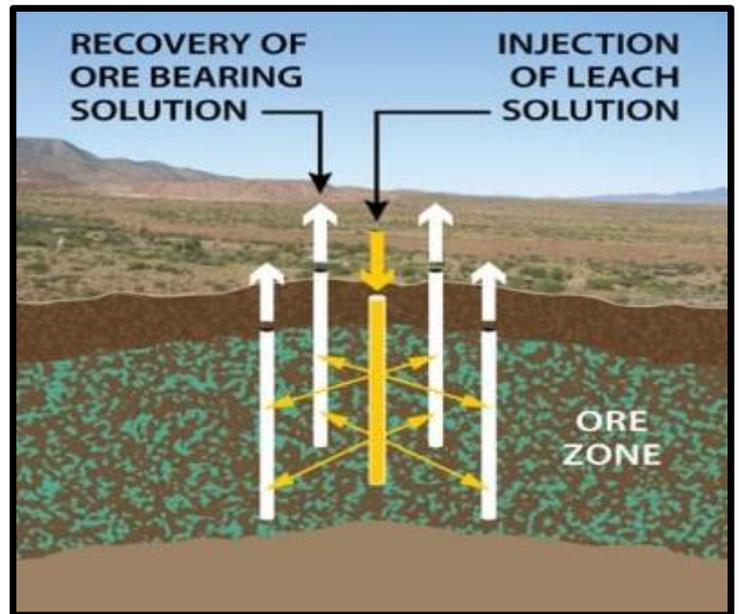
Figure 4. Schematic of Insitu Recovery process
