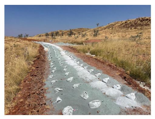
Figure 4: Drill spoil from TARC020 highlighting the significant down-hole intersection of pegmatite (in white).
