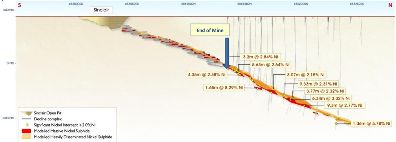
Figure 1: Sinclair Nickel deposit longitudinal projection with mine development showing mineralised Ni drill intercepts greater than 2% Ni beyond the limit of existing mine development (previously reported to ASX on 20 October 2014 – Talisman to Acquire Sinclair Nickel Project)
