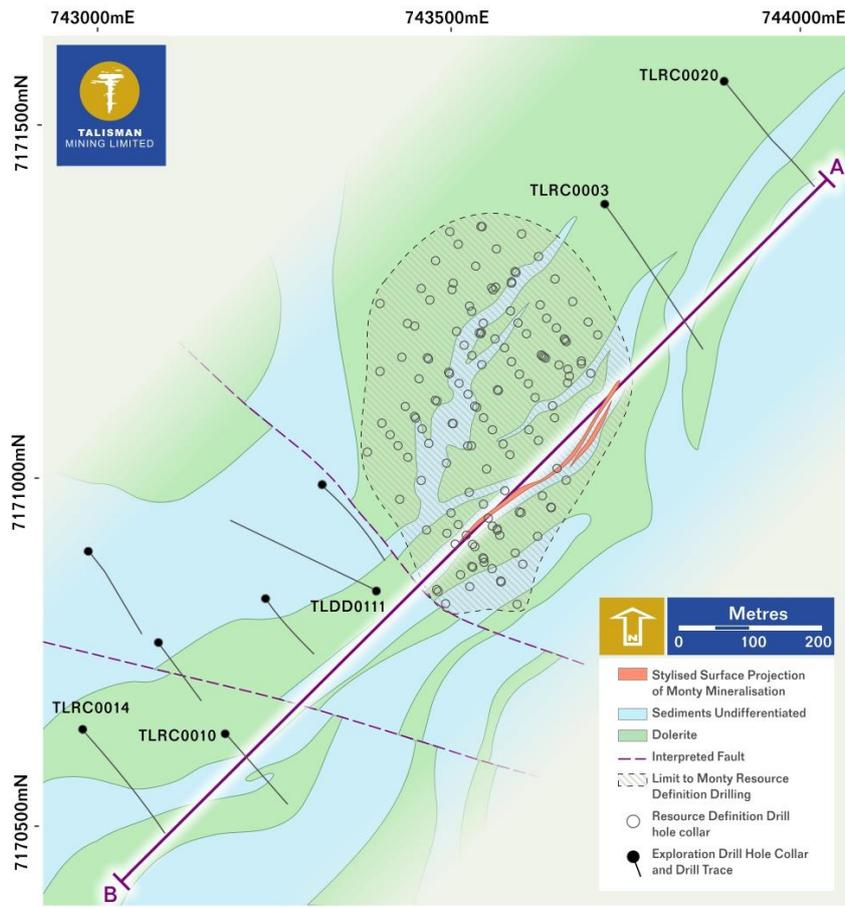
Figure 3: Plan view of Monty Resource drill collars (outlined), and Joint Venture exploration RC and diamond holes
