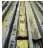
The larger diameter PQ diamond drilling was not sampled to provide a grade analytical sample, with whole core sent to AMTEC laboratories in Perth for ore processing test work.
