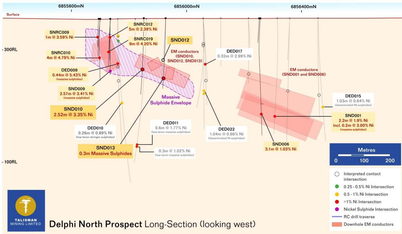
**Figure 4: Delphi North projected long section showing new and existing nickel massive sulphide intersections, newly modelled (and historic) DHEM conductors for SND010, SND012 and SND013, and an interpreted Massive Sulphide Envelope.**
