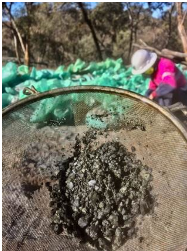
Figure 3: High-grade Cu sulphide mineralisation in RC drill chips from Blind Calf.
