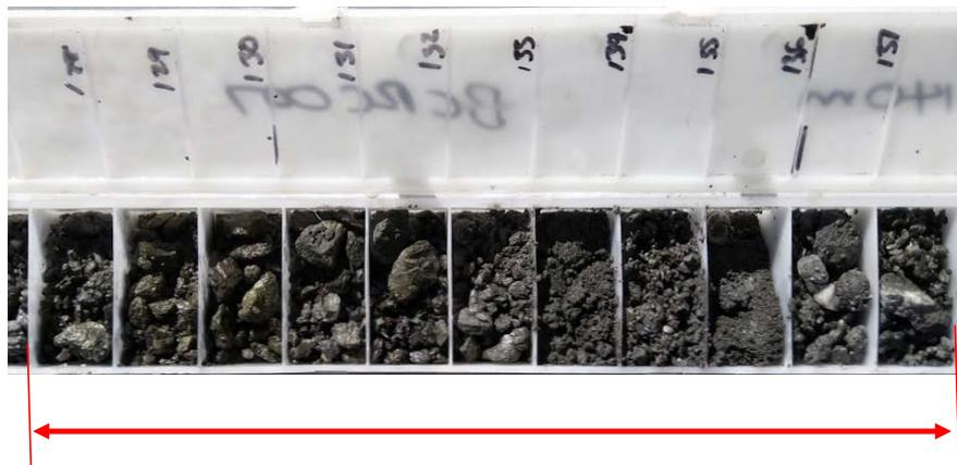
Figure 1: Blind Calf RC drill chips from BCRC007
