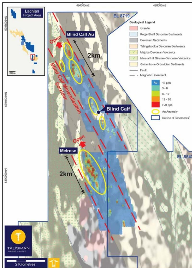
Figure 2: Blind Calf Prospect area, showing recent soil sample gold contouring over magnetics and simplified geology
