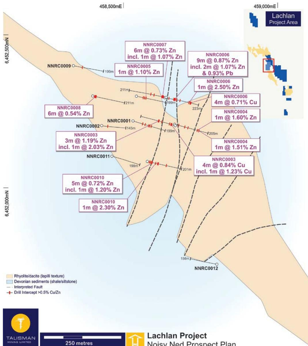
Figure 5: Noisy Ned - Drill collar locations over simplified solid geology.
