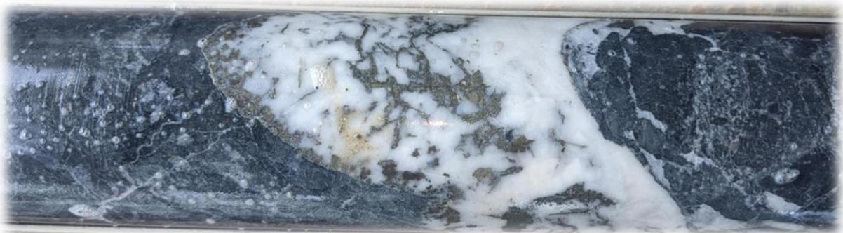
Figure 5: Core Photo showing stockwork (15cm) quartz/carbonate stringer vein containing sulphide mineralisation hosted in carbonate altered andesitic rocks.
