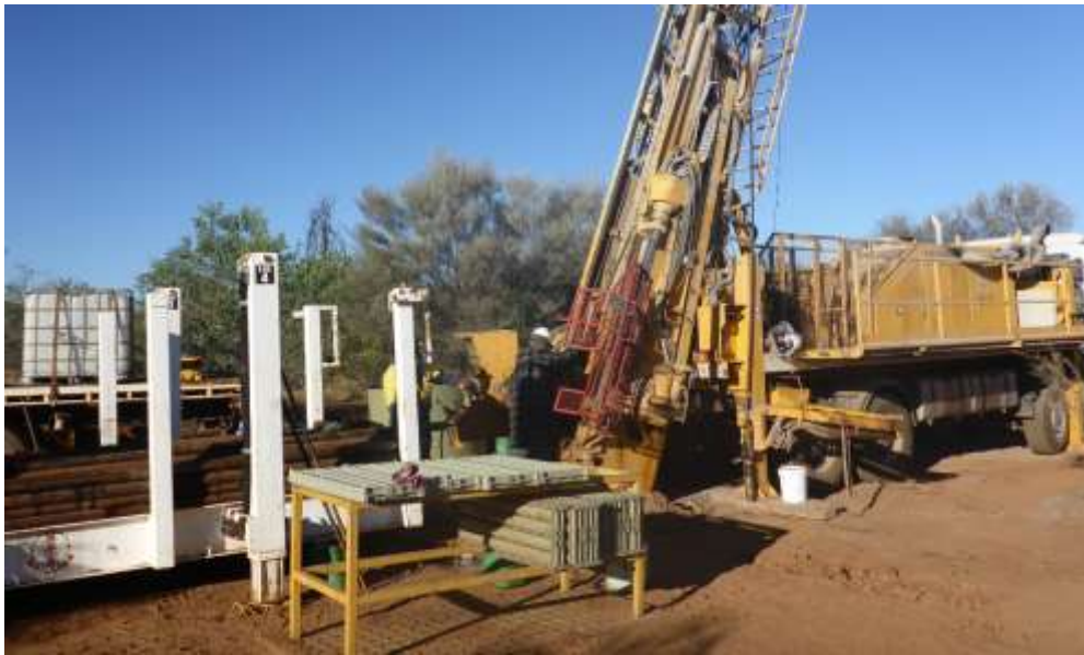
Figure 2. Diamond Drilling at EM Target #1, Mount Hardy
