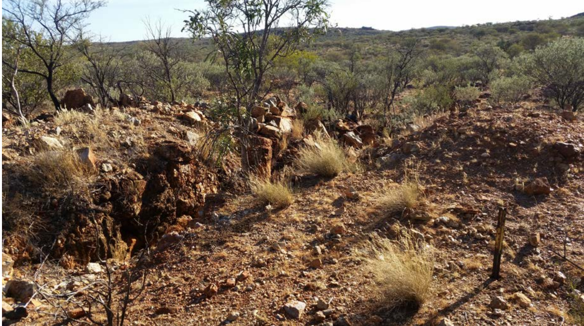
Figure 3. Photograph of the main area of workings at Bismark. Showing outcropping LCT pegmatite, historical workings and costean, and the remnants of the 1963 drill hole DDH2A (picket on right). Looking north-east towards the Clarks area.
