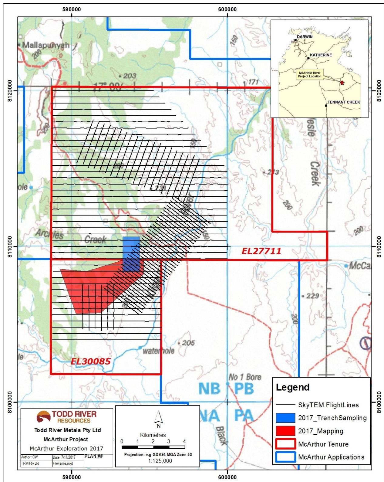
**Figure 1.** Location of the McArthur River Project, showing the area mapped, the rock and trench sampling area, The SkyTEM survey area, and adjoining new tenure. Figure 3 below covers the area outlined in the blue rectangle.
