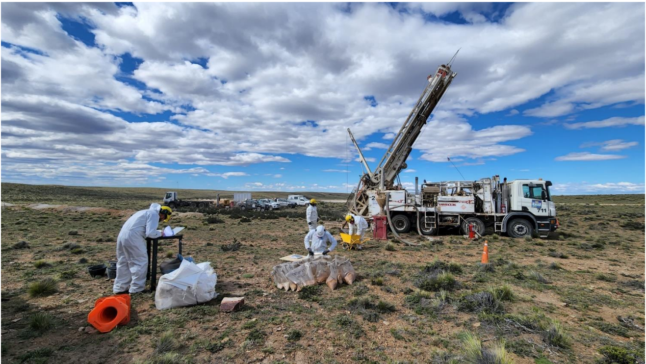
Figure 1: RC drill rig at the Karina prospect.
