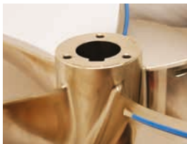
FIGURE 3: HIGH ACCURACY 5 AXIS CNC MACHINES ARE USED TO CREATE THE PATENTED 'DOVE-TAIL' GROOVE WHICH ACCEPTS THE INTERCEPTOR STRIP
