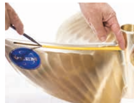
FIGURE 5: THE STRIPS CAN BE EASILY REMOVED USING HAND TOOLS. THE PROCEDURE IS SO EASY IT CAN BE DONE UNDER WATER.
