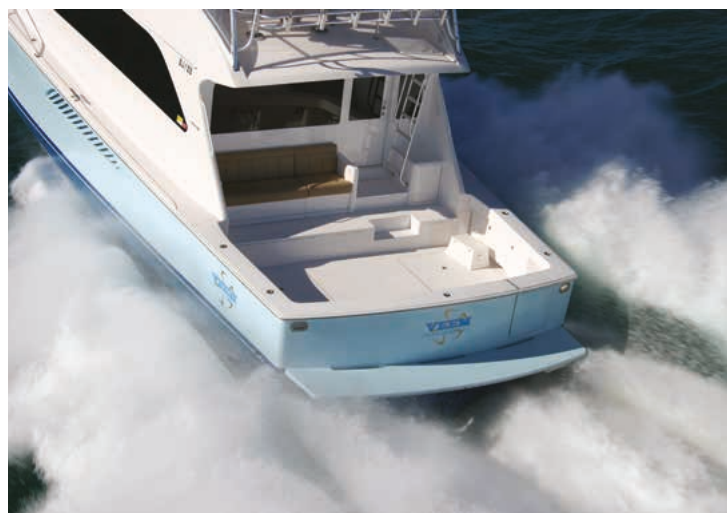
VEEM'S TEST VESSEL FITTED WITH 4,800HP TO ALLOW TESTING OF NEW PROPELLER DESIGNS UP TO 45KNOTS.
