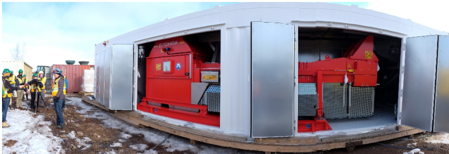
The sensor-based ore sorter that will create a rare earth concentrate delivered to the Nechalacho Rare Earth Demonstration Project in March 2021 over the winter ice road.
