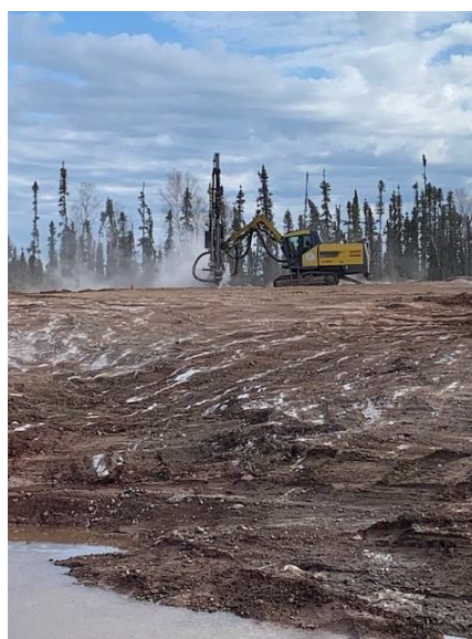
Figure 9 and 10 – Removal of overburden to rock; Drilling underway in preparation for first blast of ore.
