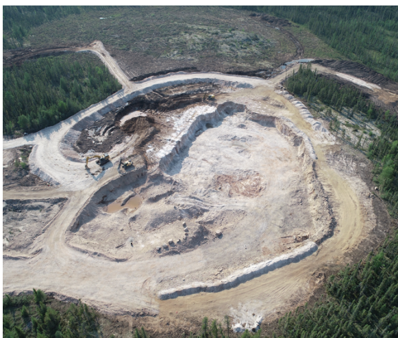
Drone image of North T pit with drilled holes ready to blast
