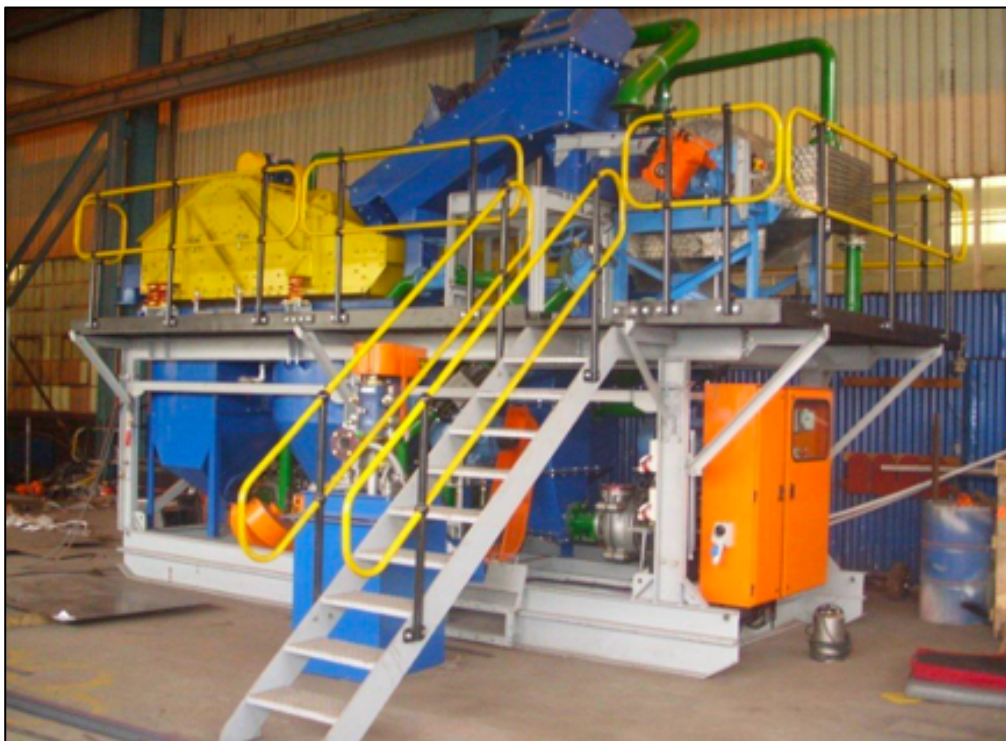
Figure 1 - A Dense Media Separator to be used in Vital's rare earth extraction process
