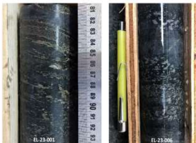
Figure 2: examples of the sulphide mineralisation intersected in holes EL-23-001 and EL-23-006, as labelled. See Announcement dated 17 April 2023 for more details
