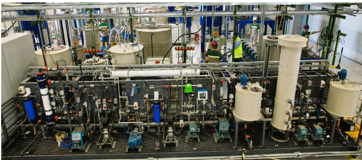
Figure 7: Spent Solution and Water Treatment Package: designed to enable complete recycling of process water, and regeneration of Ammonium Bicarbonate into Ammonium Sulphate.
