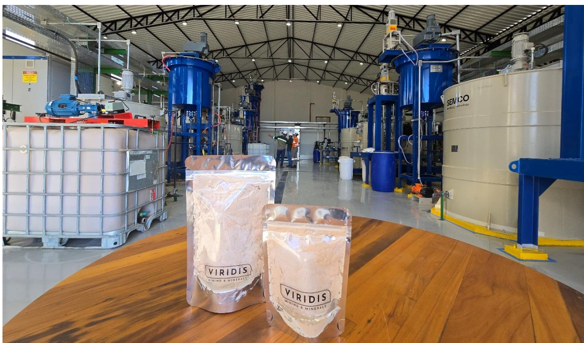
Figure 1: First production of MREC from the Demonstration Plant. At nameplate capacity, ~8kg of MREC is produced per day, providing sufficient volumes for internal laboratory verification and supply to potential offtake partners.
