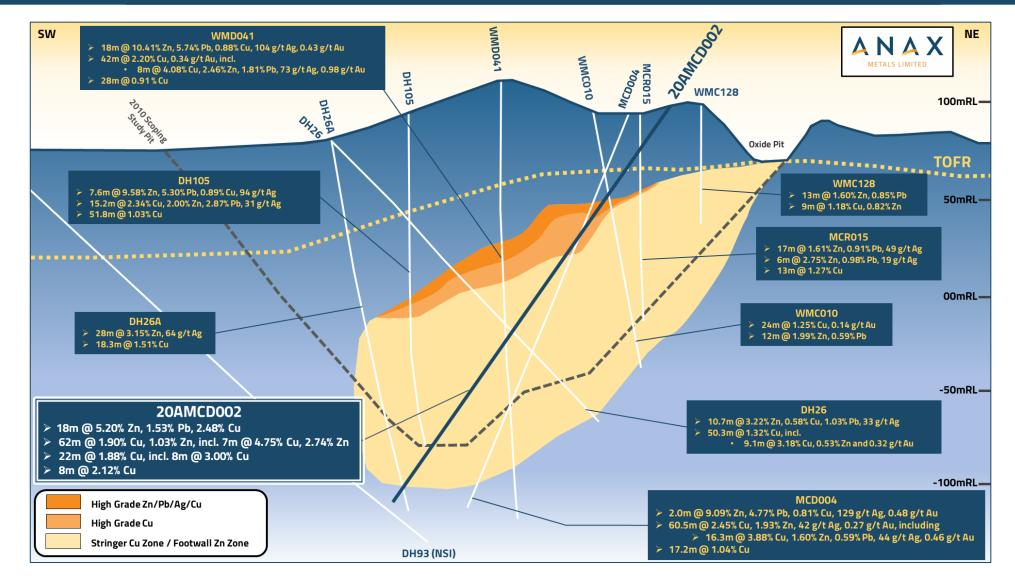
*Figure 3: Mons Cupri Oblique Section showing 20AMCD002 and select previous drill holes.* Note: A number of holes have been omitted from the section for ease of display; only the most significant intervals are displayed - for a full list of intersections refer to Table 2 and Table 10.
