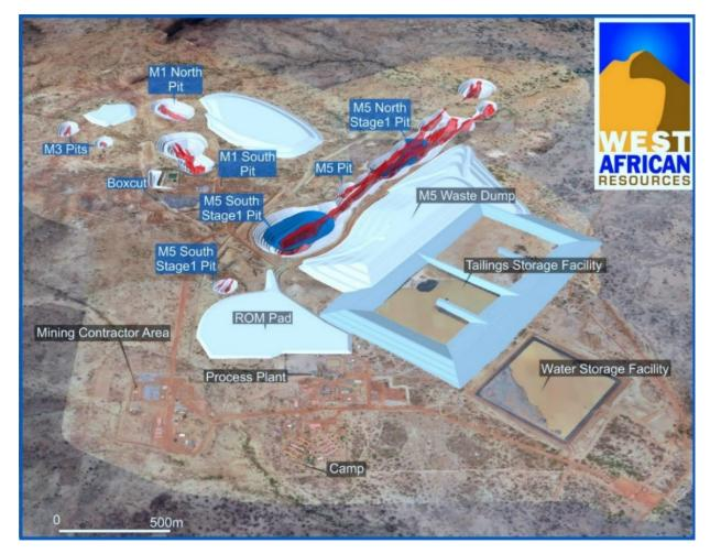
Figure 2: Sanbrado Gold Operation Layout
