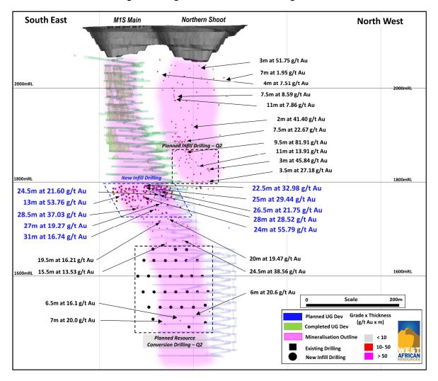
Figure 2: Long Section of M1 South Underground
