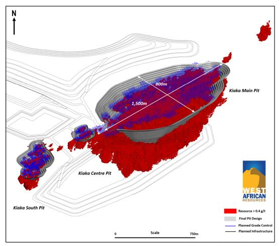
**Photo 5: Grade Control Drilling at Kiaka**
