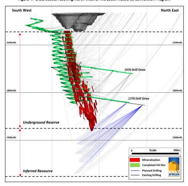
Figure 4: Cross Section Looking North West of M1 South Resource Conversion Program
