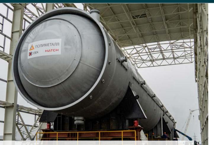
Polymetal recently installed this autoclave at their second Pressure Oxidation Plant (POX-2) in Amursk, Russia.
