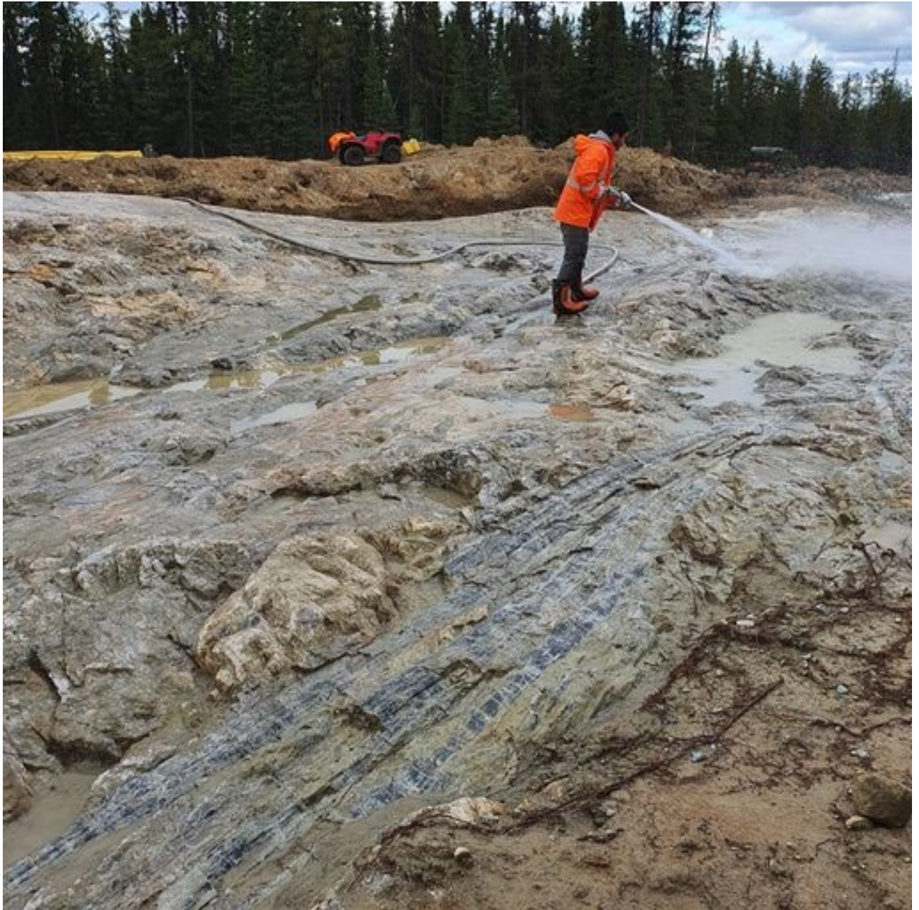
Figure 5: North-East view of main dyke at Cancet showing spodumene crystals exposed during stripping
